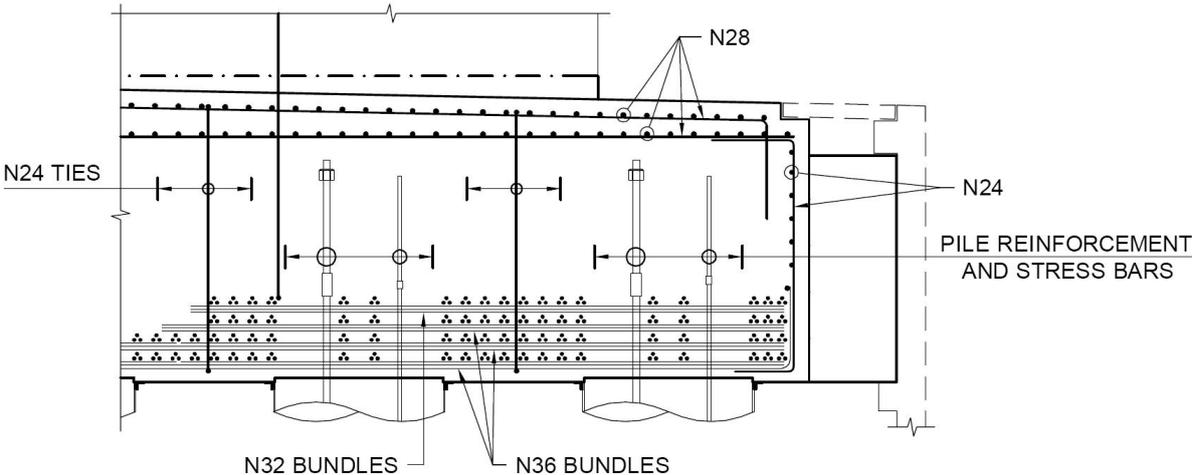
**Figure 6 – Part Cross Section Through River Pier Pilecaps**
