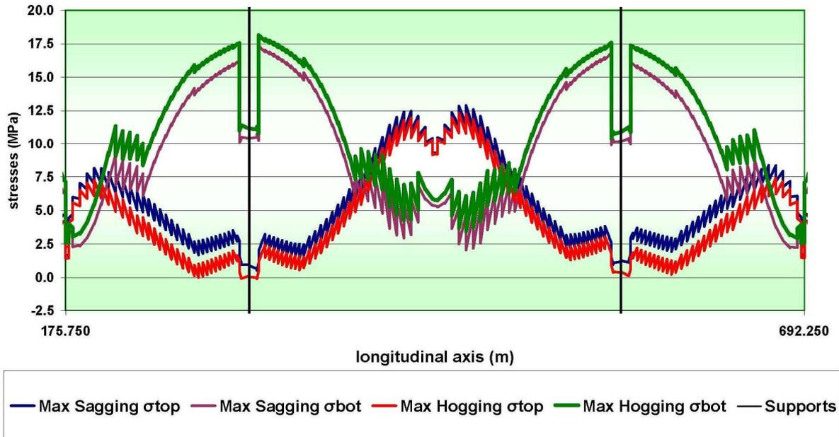
**Figure 8 – Permanent Dead Load Stresses in the Superstructure**
