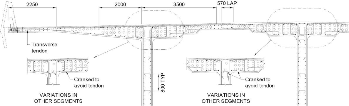
**Figure 9 – Typical Box Girder Top Flange Details**
