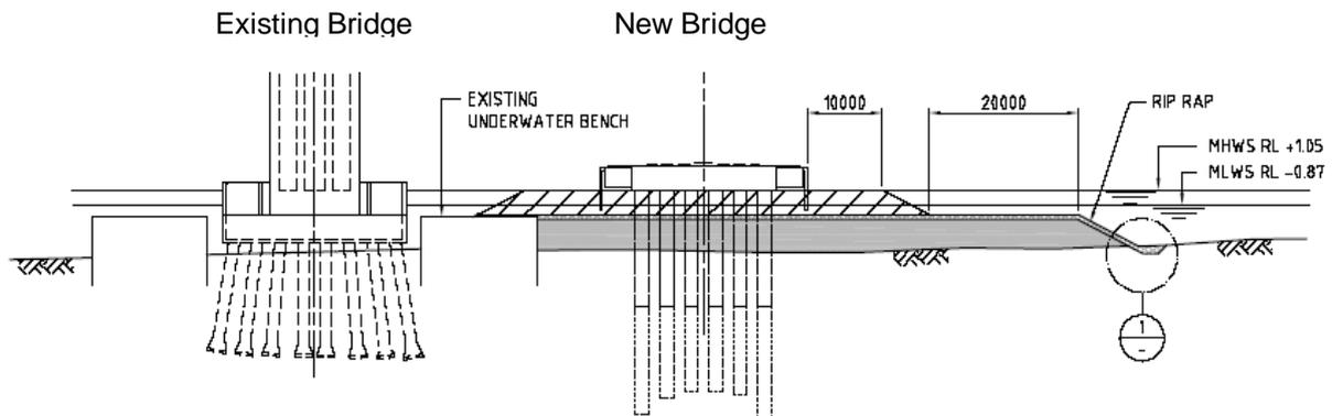
**Figure 5 – Cross Section through Pier 6 Ship Arrestor Island**
