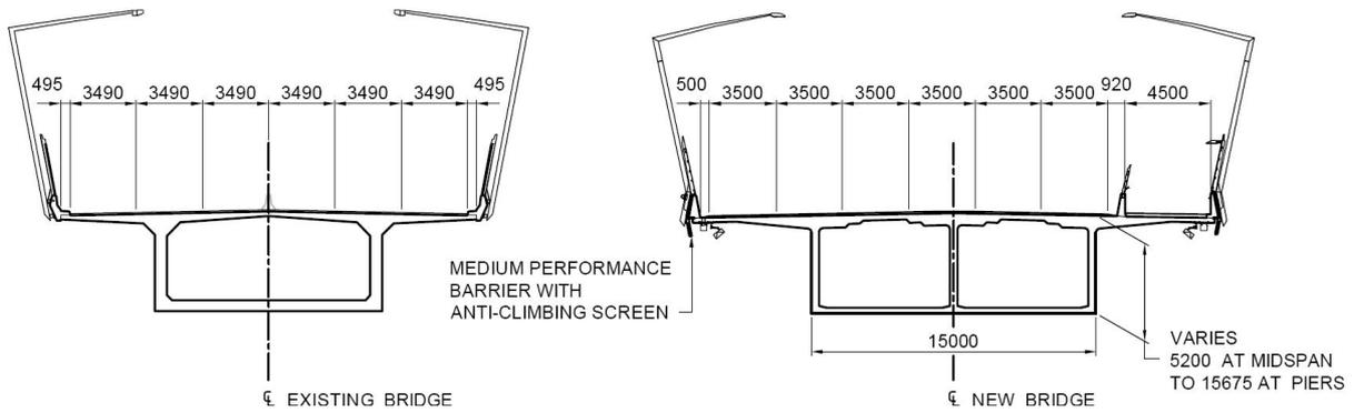
**Figure 2 – Main Span Cross Section**
