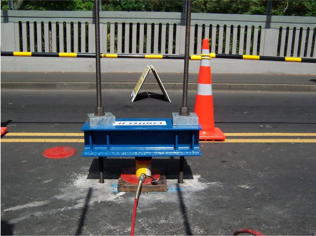
Figure 7 – Load Test Equipment Above Deck
