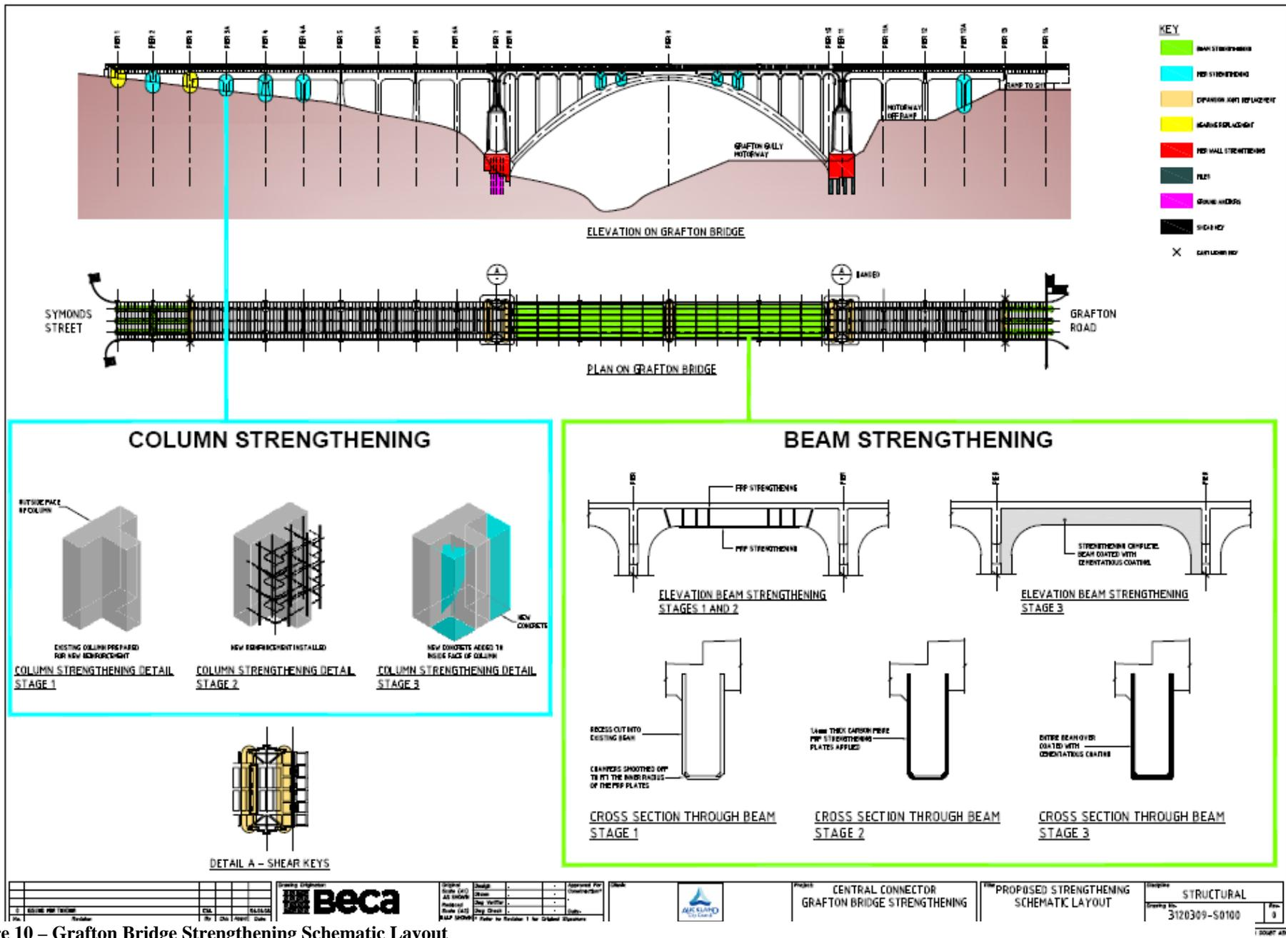
Figure 10 – Grafton Bridge Strengthening Schematic Layout
