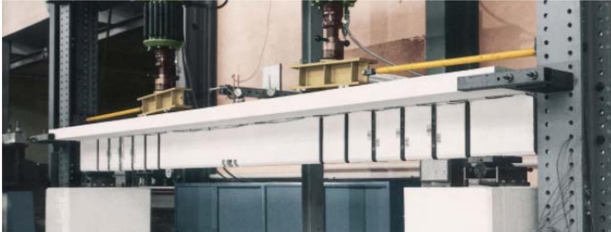
Figure 9 – Laboratory Testing of FRP Shear Strengthening
