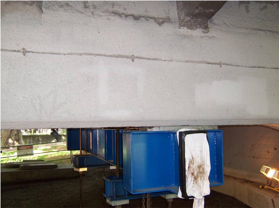
Figure 8 – Load Test Reaction Beam Below Deck
