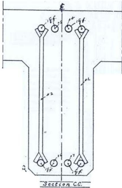
Figure 5 – Shear Bar Drawing
