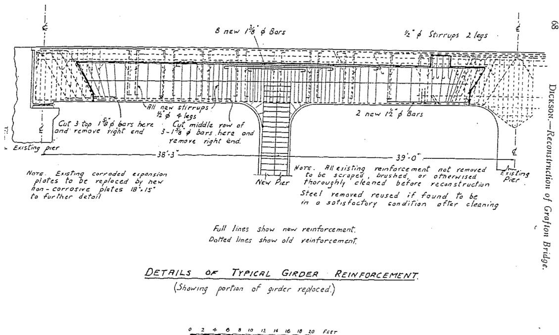
Figure 3 – 1936 Reconstruction Drawing of New Pier and Replacement Beams
